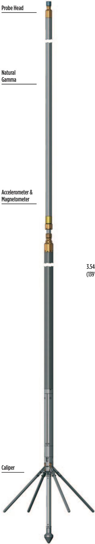
Borehole Geometry Probe
